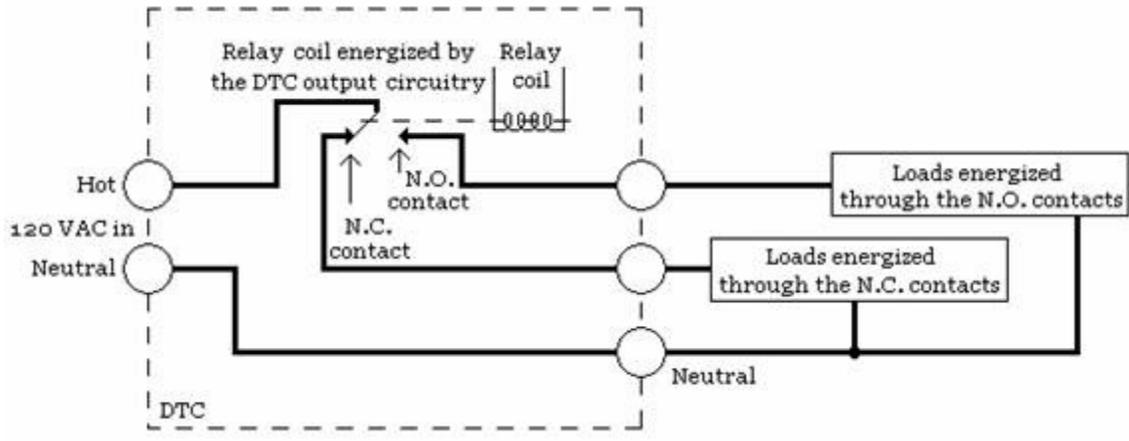
DTC Relay Closure Output Wiring
